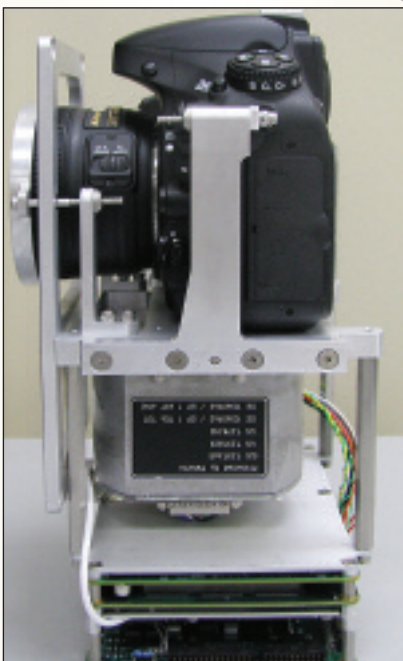
Applanix direct mapping solution for larger UAVs: from top to bottom, camera, inertial sensor, GNSS receiver.
