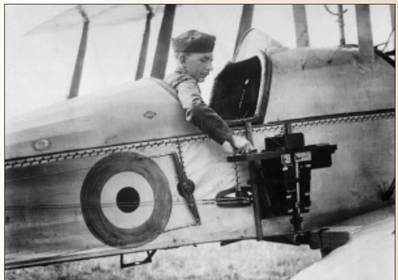
A sergeant of the Royal Flying Corps demonstrates a C type aerial reconnaissance camera fixed to the fuselage of a BE2c aircraft, 1916. Credit Imperial War Museum's Catalogue Number Q33850 ( http://www.iwm.org.uk/collections/item/object/205193165 )
