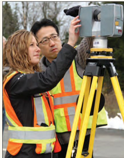
Figure 6. Alice and Yong-Won entering data collection parameters into the laser scanner.
