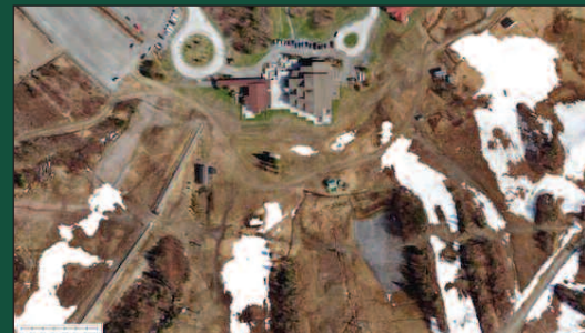
Figure 1 - A sample of an orthomosaic of Marble Mountain, Newfoundland, composed of 142 aerial photos collected by a SenseFly eBee RTK mapping drone operated by UKKO, a division of Ag Business & Crop Inc.
