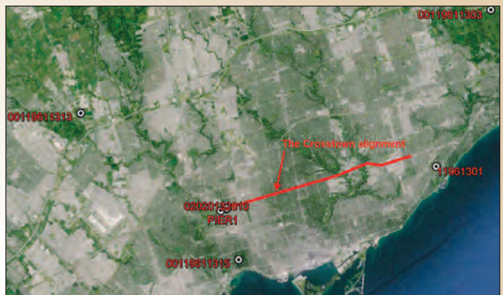
Fig. 4 – The Eglinton Crosstown LRT alignment and framework points used for the transformation
