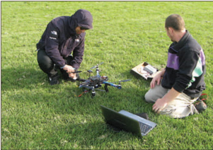
York University students Sonal Ranjit, Earth Science (left) and Dennis Sherman, Geomatics Engineering (right) testing the ArduCopter 3DR DIY 2014 Quad small unmanned aerial mapping system.
