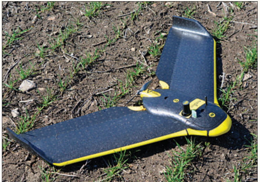
The SenseFly eBee UAV with On-Board RTK Survey Accuracy GPS Location Capability.
