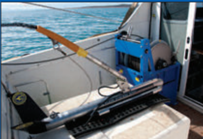
Parks Canada side-scan sonar towfish, cable and winch on the CHS survey launch Kinglett in 2010. Photo credit: Jonathan Moore, Parks Canada
