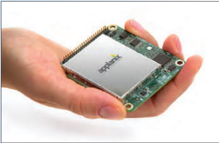
The Applanix APX-15 UAV board for small UAVs
