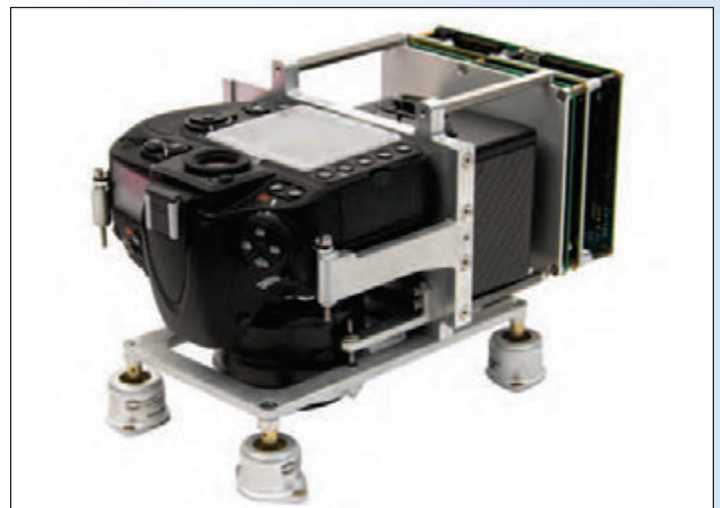
An RGB camera based Direct Mapping Solution (DMS) payload for medium-sized fixed-wing UAVs
