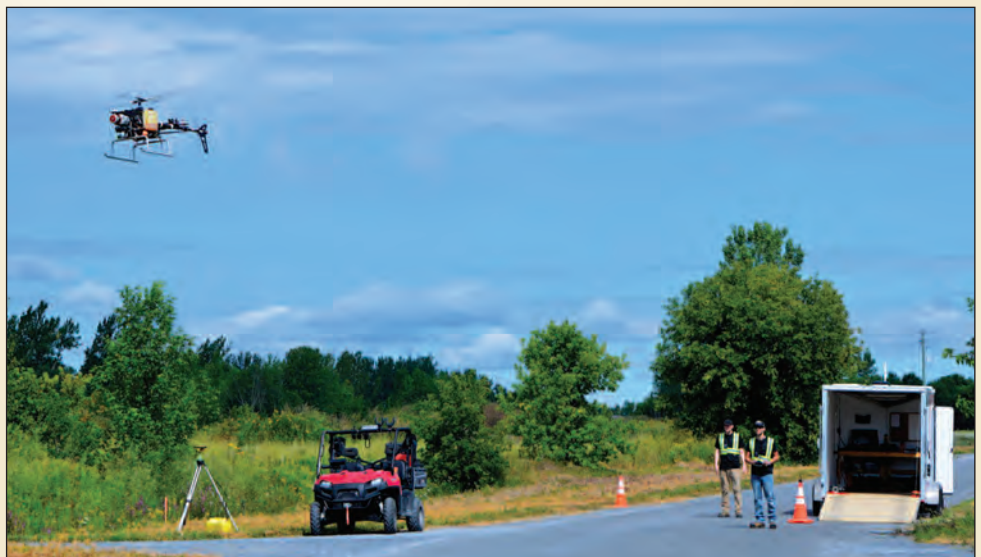
RME Geomatics Inc. staff Morgen Parks and Matt Peschisolido launch the custom-designed Renegade UAV on a combined LiDAR/aerial photography mission.
