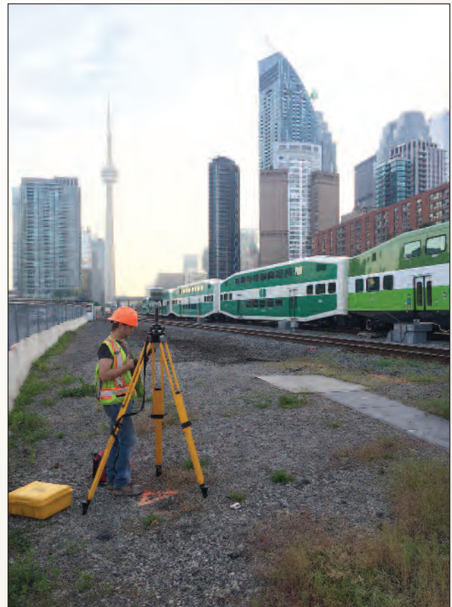
Nic Hinsperger setting Control for the Mobile LiDAR Survey
