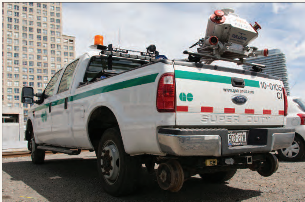
Tulloch's Mobile LiDAR System mounted on a GO Transit Hi-Rail Vehicle
