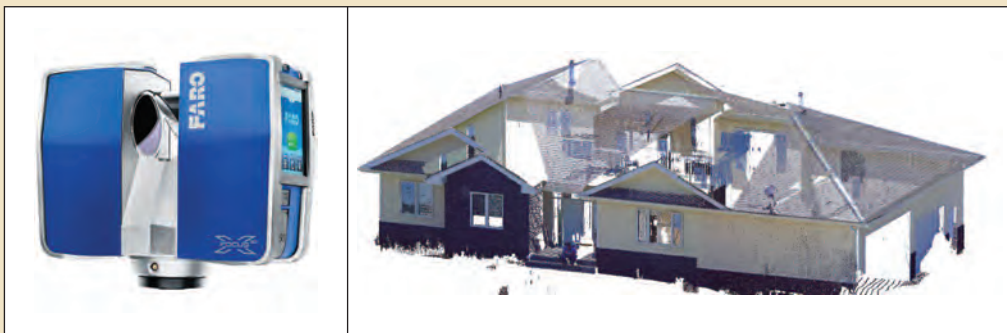
Figure 2: FARO Focus3D X 330 and scanning point cloud
