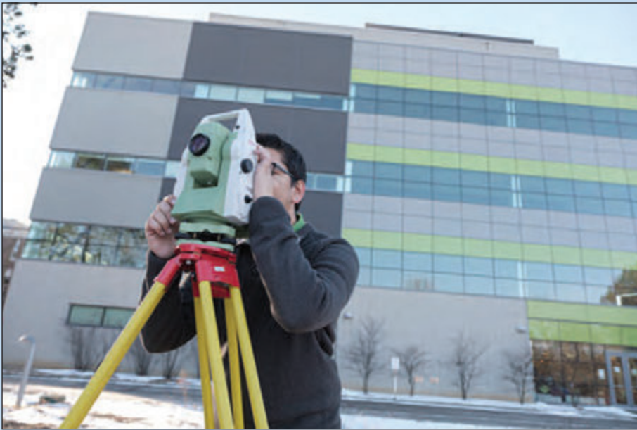
Environment student Aujas Bandlish uses a total station, an electronic/optical instrument used for surveying and building construction, as part of his Geomatics fieldwork.
