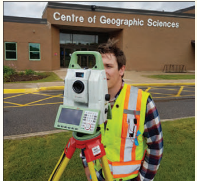
Dylan MacDonald using the Leica Nova M560 Multistation – Scanner/Robotic Total Station
