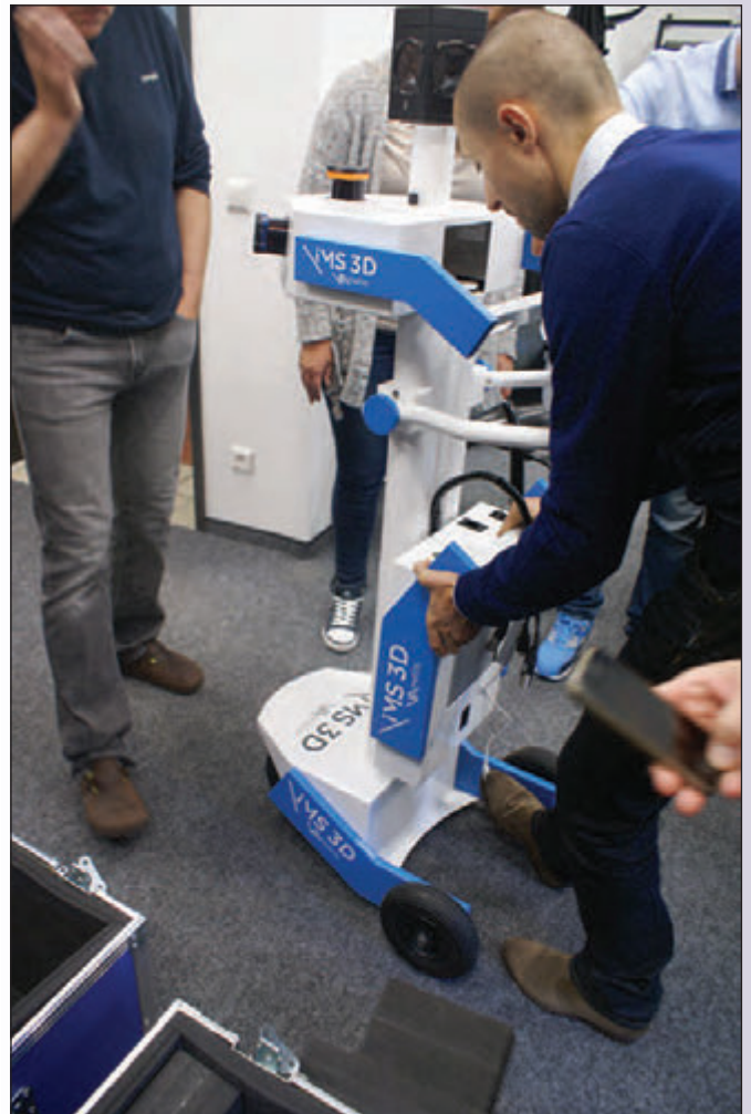
iMS3D: Jerome Ninot, president and founder of VIAMETRIS, demonstrating the iMS3D collecting 3D point clouds and 360° images with centimetre accuracy at walking speed. The iMS3D captures up to 500,000 sq. ft. per day and calibrates imagery with point cloud data even in GNSS-denied areas using SLAM technology.
