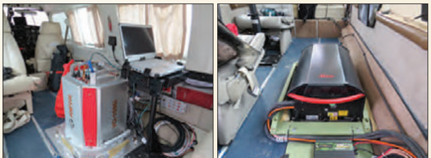
Riegl and Leica Sensors installed in fixed wing aircraft
