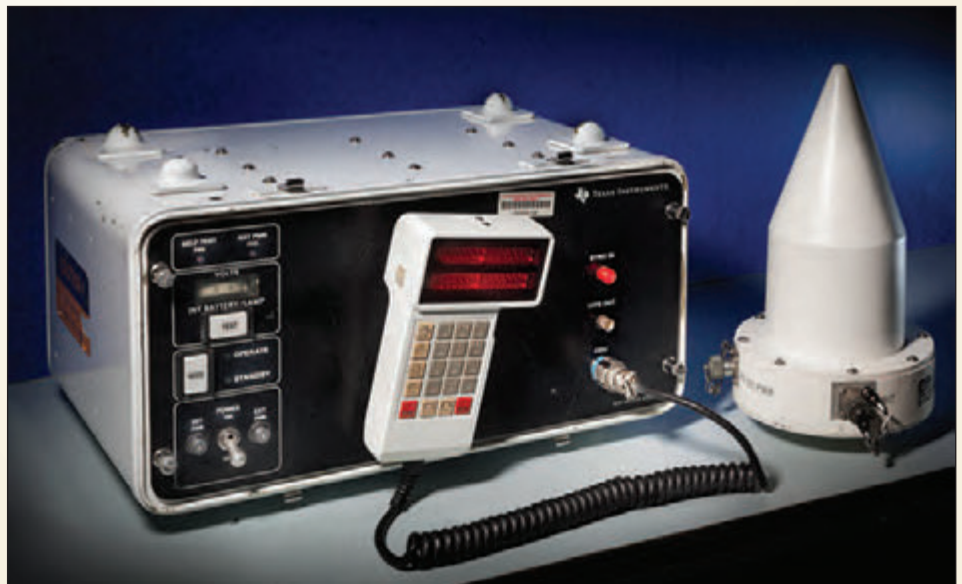
Figure 1: TI-4100 GPS Receiver - The portable Texas Instrument 4100 was the work horse of GPS field surveys in the early 1980's.
