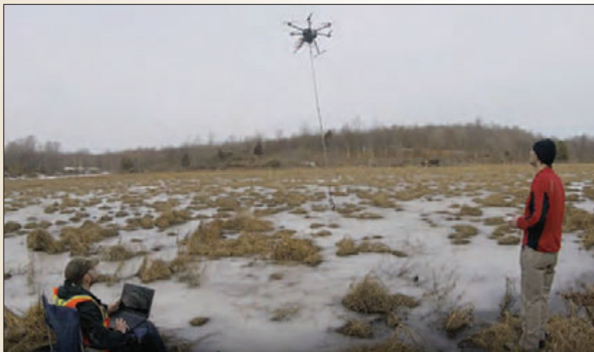
PhD student Callum Walter and Dr. Braun testing the UAV with suspended magnetometer system at the Queen's University Biological Station.
