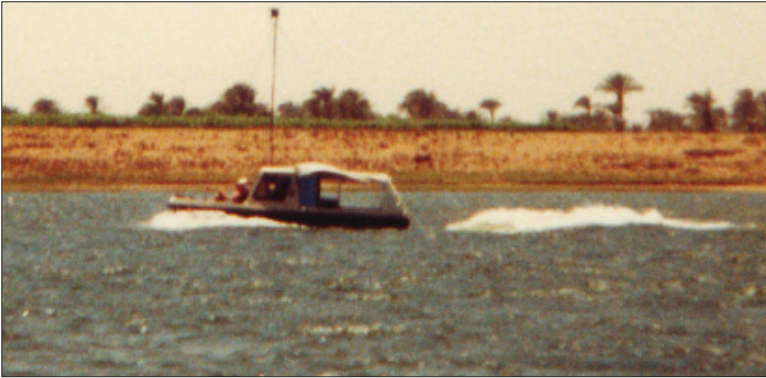
Shallow draft water jet propelled survey launch on the Nile
