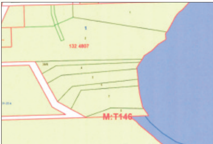
Figure 3 - An equitable apportioning of accretion (note the bends in the side bounds)
