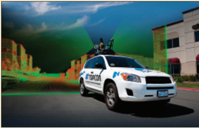
Mobile Mapping System (Topcon IP-S2) collecting 3D data on city streets
