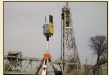
Terrestrial LiDAR System (Topcon GLS-1000) being used to survey bridge
