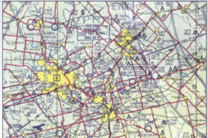
Figure 1: Clip of a Visual Navigation Chart (VNC) used by manned aircraft to navigate the 3D airspace and includes hazards such as glider operations and towers.
