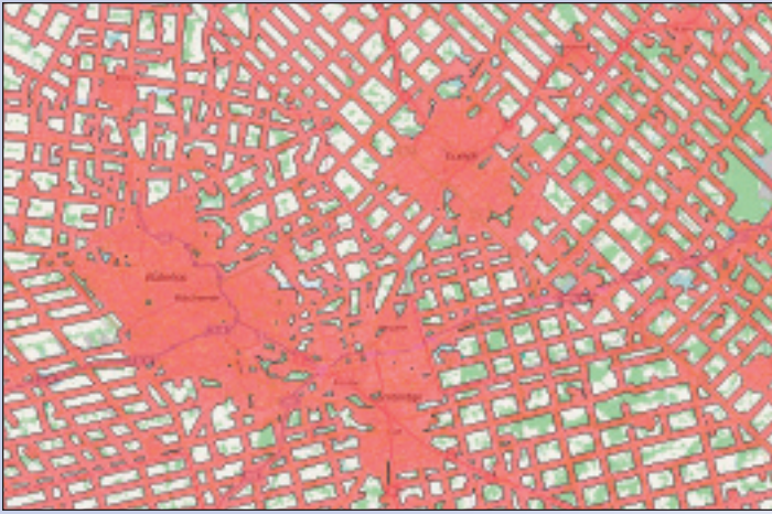
Figure 2: Clip of same area as Figure 1 showing areas of potential UAV deployment challenges due to road restrictions.
