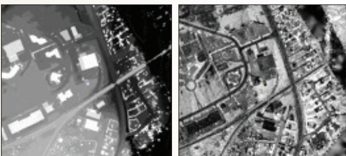
Figure 4: LiDAR digital surface model (DSM) (Left); LiDAR intensity georeferenced image (Right)
